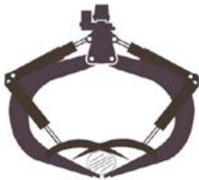
Grapple with hydraulic clamping arm
