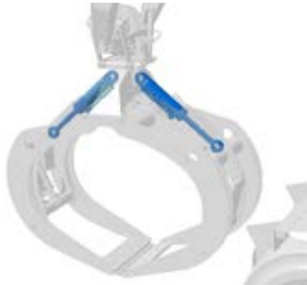
Grapple with hydraulic clamping arm
